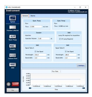
ASTRA's HPLC DASHBOARD™ provides the convenience of a handheld controller with real-time indication and setup of your HPLC system.
