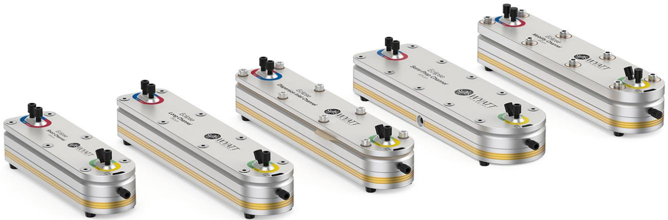
Left to right: Short, Long, Dispersion Inlet (variable-height), Semi-Prep and Mobility fixed-height channels
