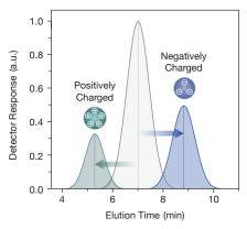
In EAF4, the zero-field retention time (grey peak) is determined by the particle's hydrodynamic radius. Application of an electric field to the EAF4 channel shifts the retention time according to the sign and magnitude of the particle's charge.
