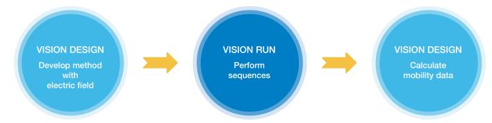
EAF4 workflow with VISION™. VISION DESIGN calculates the expected shift in elution time due to applying electric and cross-flow fields in the Mobility Channel, to a sample with a given size and charge. VISION RUN performs the set of experiments and stores the data in a single file. VISION DESIGN automatically processes the complete series of experiments, calculating size, mobility, zeta potential and charge.
