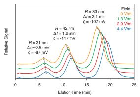
The shift in retention time due to the electrical field is analyzed automatically to determine zeta potential and electrophoretic mobility of each eluting peak. Shown here is the analysis by EAF4 of a mixture of three polystyrene nanoparticles, resulting in both size and zeta potential determination of each component.
