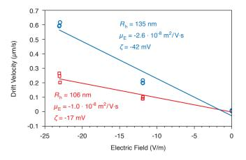
VISION DESIGN automatically calculates the size, mobility, net charge and zeta potential for both populations. The measurement reveals a 2.5 fold difference in zeta potential.
