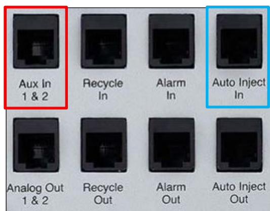
a) Auxiliary signal port (red) and auto inject signal port (blue) location on the rear panel of the microDAWN (NEON™) MALS detector. The older versions, i.e. \mu DAWN™ MALS detector (serial number xxxx-UD) have two Aux In ports (Aux In 1&2 and Aux In 3&4).
