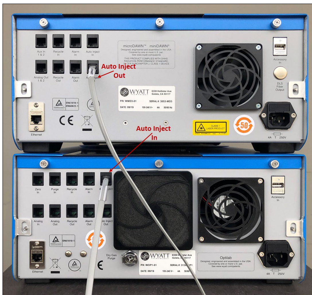
Figure 6: An autoinject crossover cable connection between the microDAWN (NEON) MALS detector (top) and microOptilab detector or Optilab detector (NEON) (bottom) for optimized synchronization. The crossover cable transmits the autoinject signal received by the light scattering detector to the RI detector for optimized synchronization.
