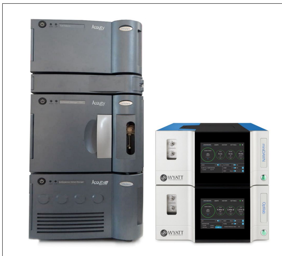
Figure 1: Example of an ACQUITY UPLC system with Wyatt instrumentation. Note that the Waters components, column oven, optical detectors, and Wyatt detectors are stacked and the Wyatt instruments are on the left of the ACQUITY UPLC system to help minimize the tubing length. Short tubing minimizes delay volumes and maintains the chromatographic resolution. No tubing connections are present in this image.
